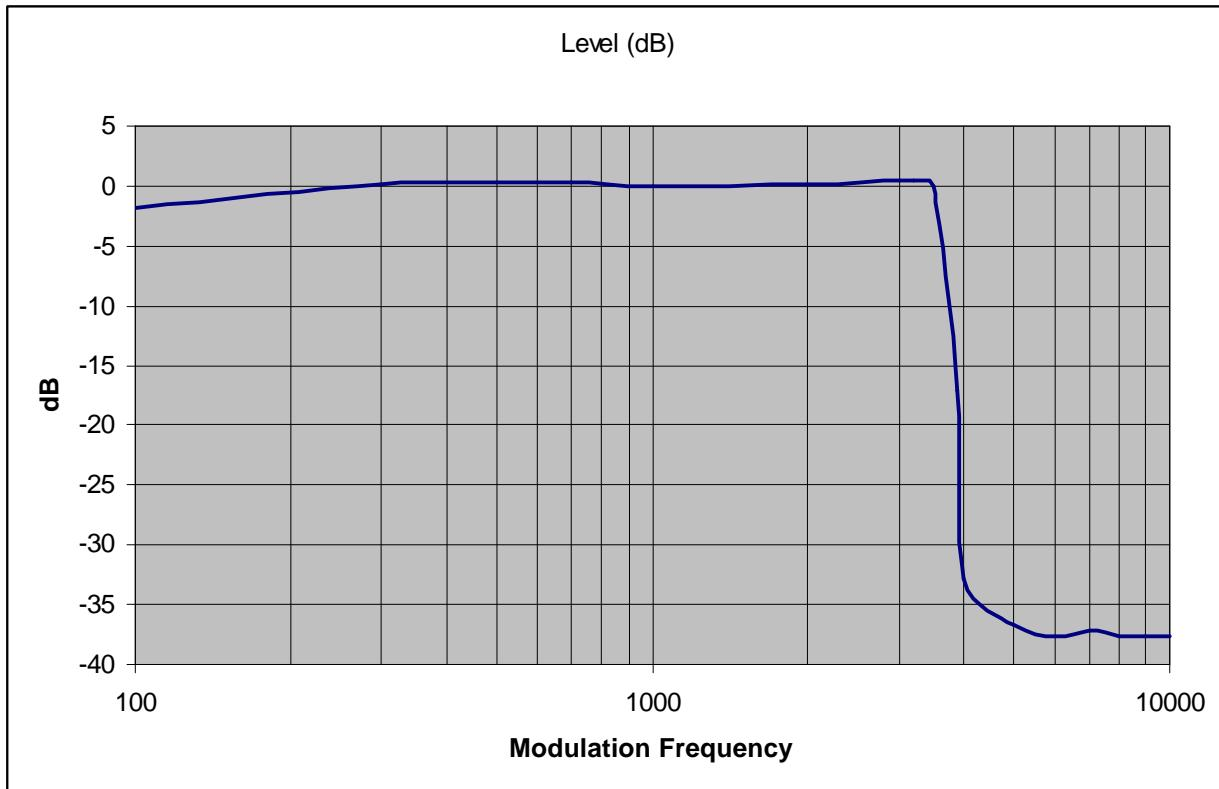
Modulation Characteristics – 47 CFR 2.1047 (b)
