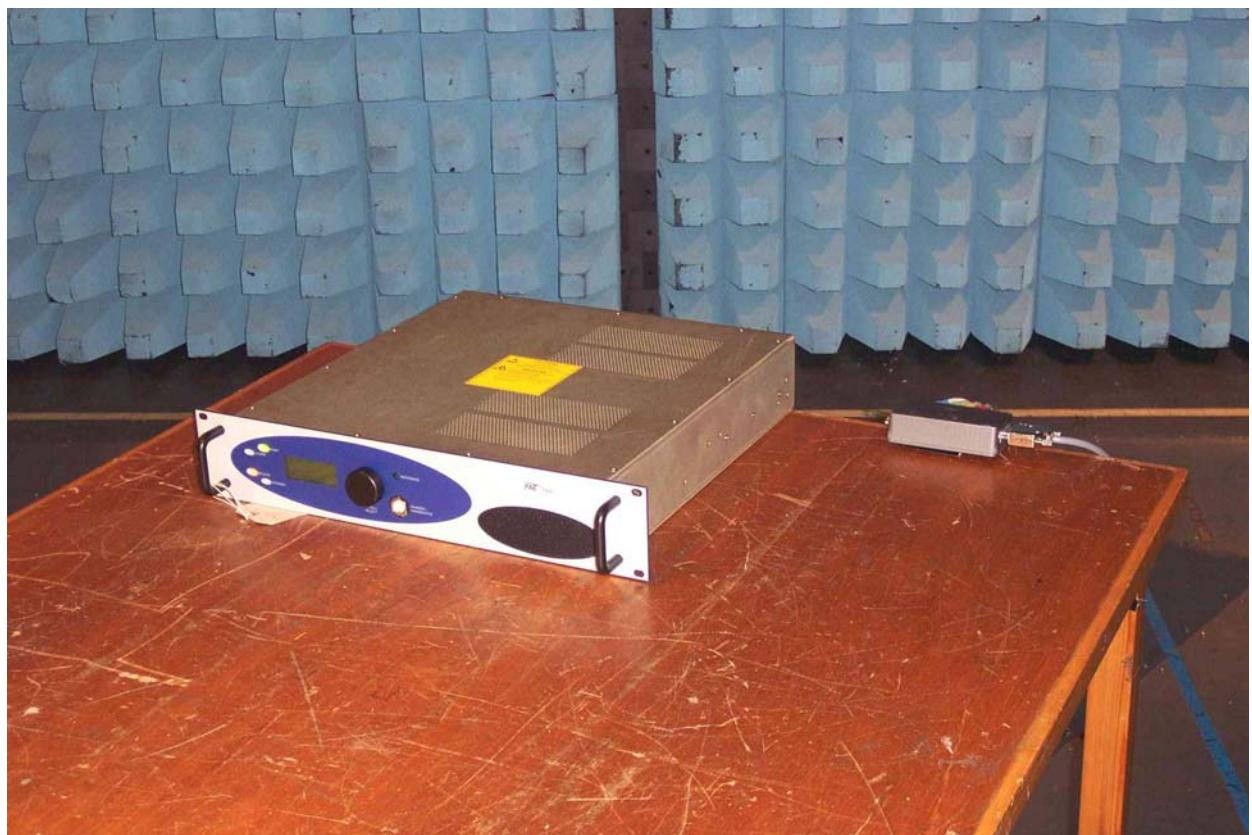
**Conducted Emissions Test Set Up (T6R)**
