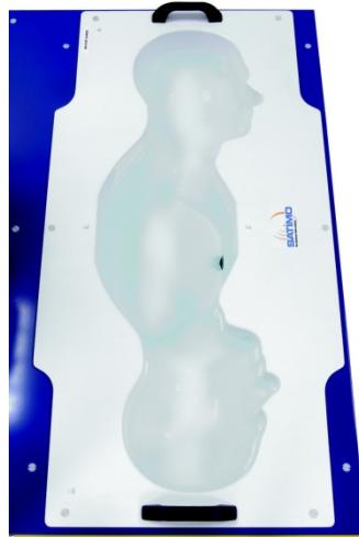
The bottom plate contains three pair of bolts for locking the device holder. The device holder positions are adjusted to the standard measurement positions in the three sections. A white cover is provided to tap the phantom during off-periods to prevent water evaporation and changes in the liquid parameters. On the phantom top, three reference markers are provided to identify the phantom position with respect to the robot.
