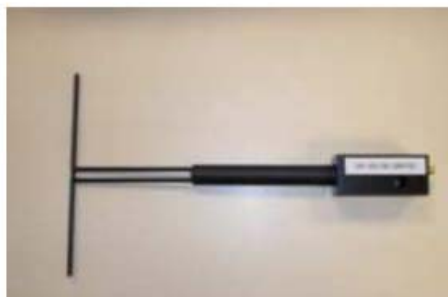
Figure 1 – Satimo COMOSAR Validation Dipole
