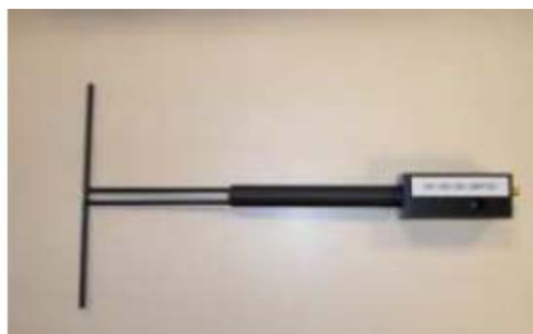
Figure 1 – Satimo COMOSAR Validation Dipole
