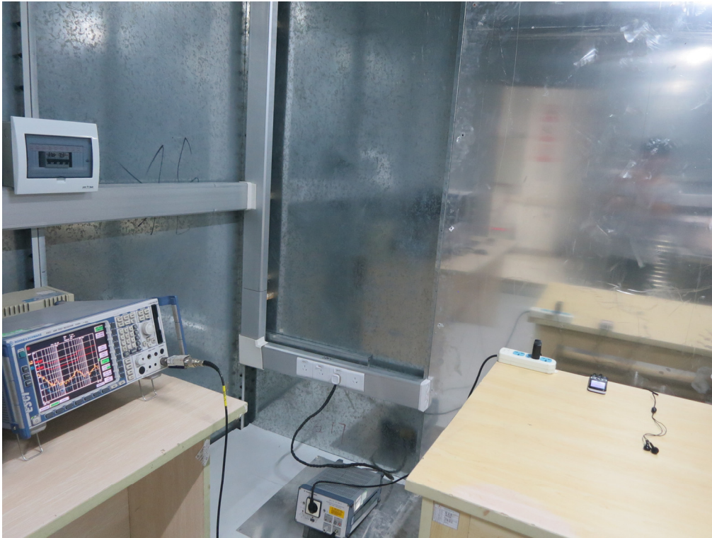
FCC RADIATED EMISSION TEST SETUP
