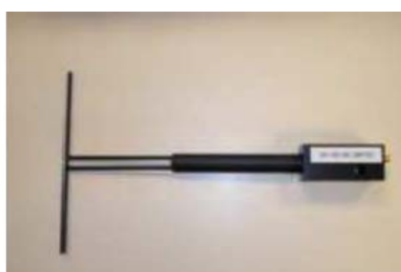
Figure 1 – Satimo COMOSAR Validation Dipole
