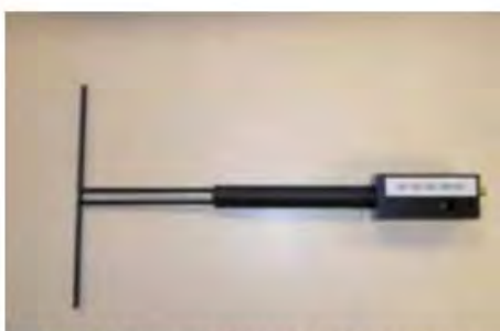
Figure 1 – Satimo COMOSAR Validation Dipole
