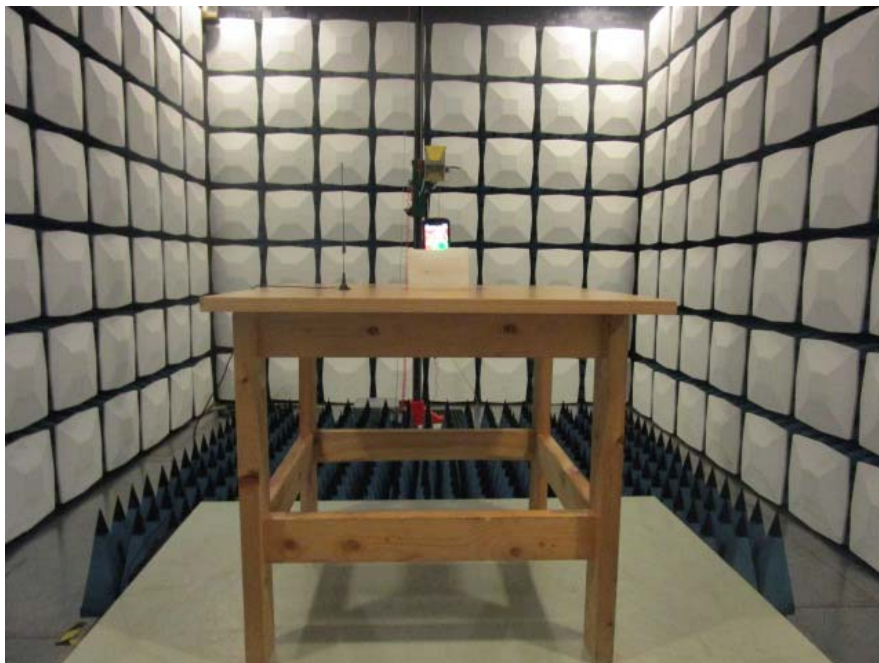
Radiated Emission View---Above 1GHz
