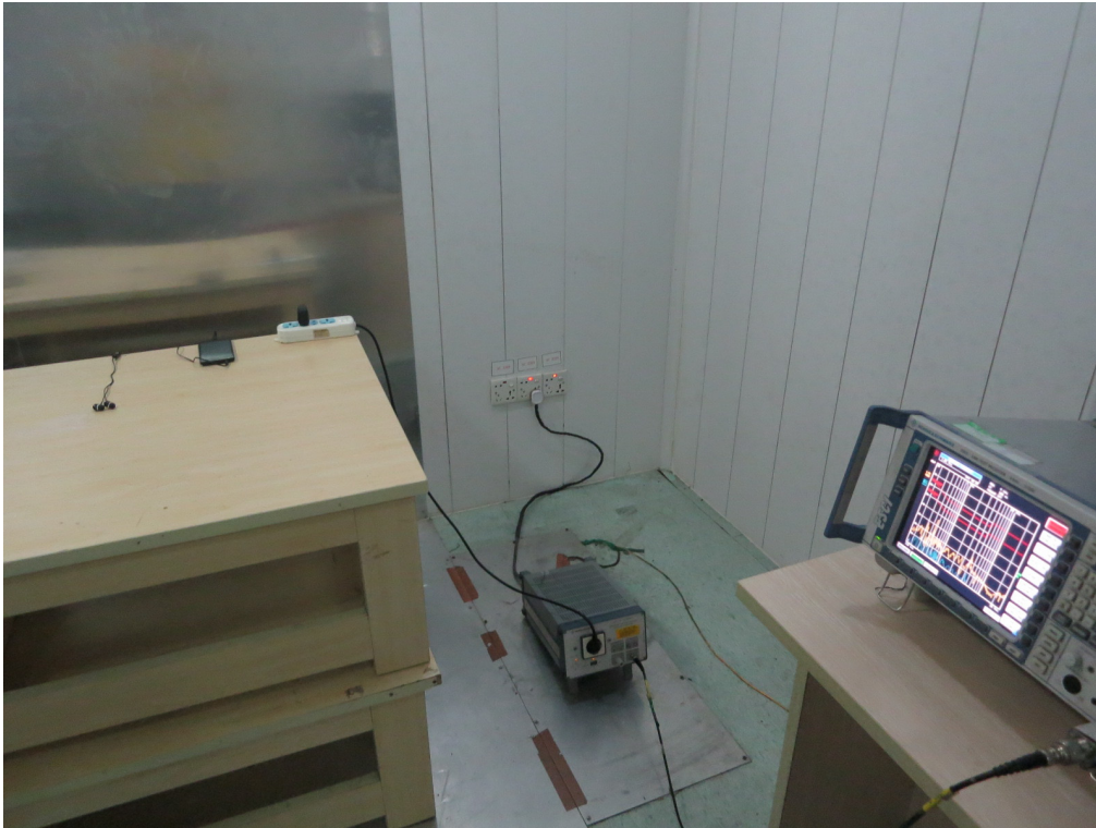
FCC LINE CONDUCTED EMISSION TEST SETUP
