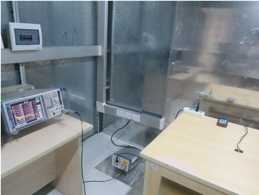
FCC RADIATED EMISSION TEST SETUP
