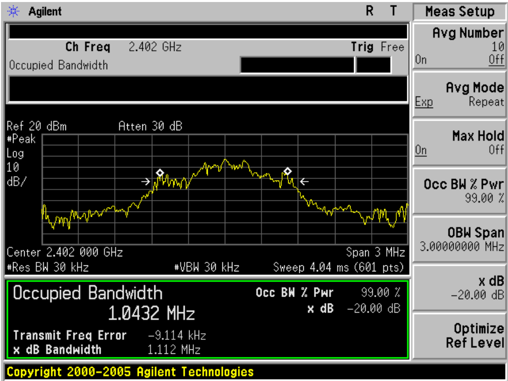
TEST PLOT OF BANDWIDTH FOR LOW CHANNEL
