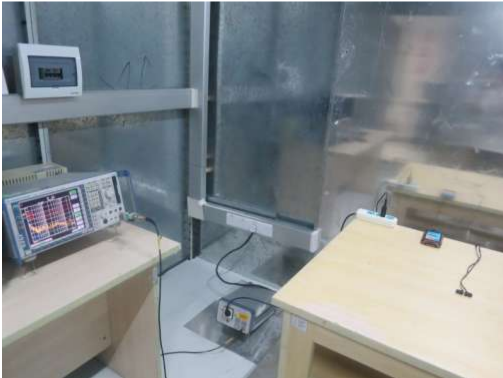
FCC RADIATED EMISSION TEST SETUP
