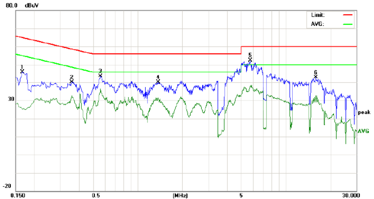
Line Conducted Emission Test Line 1-L
