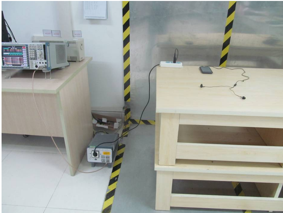
FCC LINE CONDUCTED EMISSION TEST SETUP
