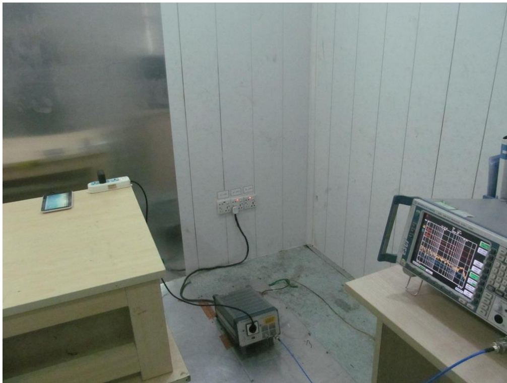
FCC RADIATED EMISSION TEST SETUP
