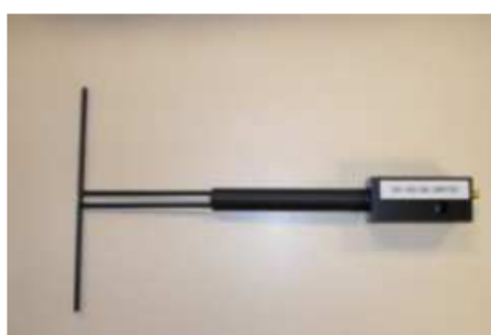
Figure 1 – Satimo COMOSAR Validation Dipole
