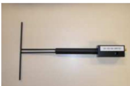
Figure 1 – Satimo COMOSAR Validation Dipole
