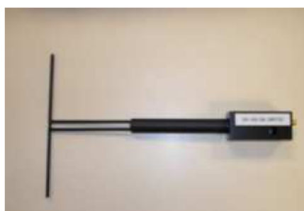
Figure 1 – Satimo COMOSAR Validation Dipole
