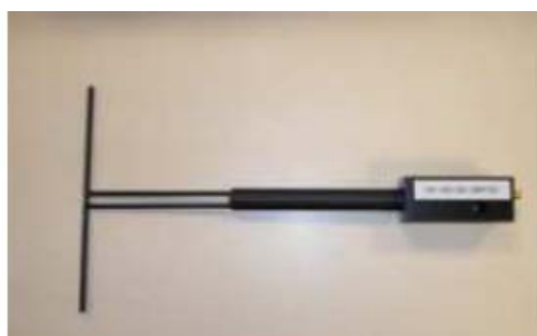
Figure 1 – Satimo COMOSAR Validation Dipole
