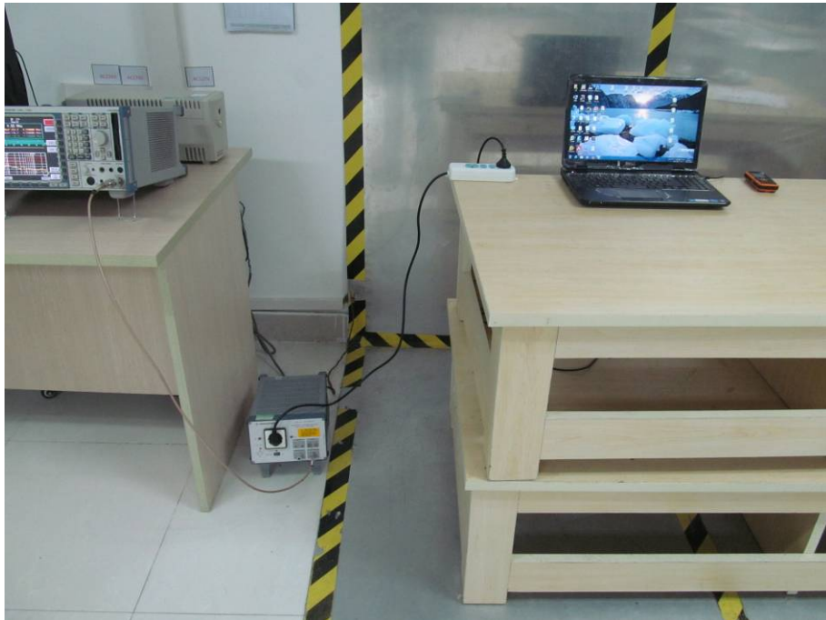
FCC LINE CONDUCTED EMISSION TEST SETUP
