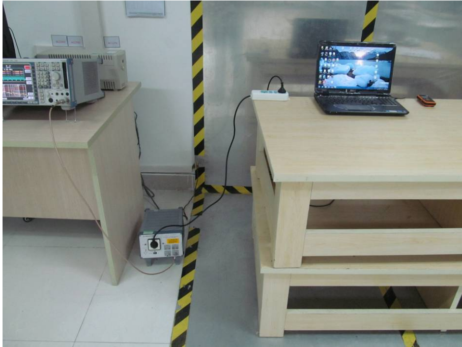
FCC LINE CONDUCTED EMISSION TEST SETUP
