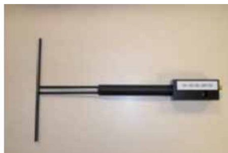
Figure 1 – Satimo COMOSAR Validation Dipole
