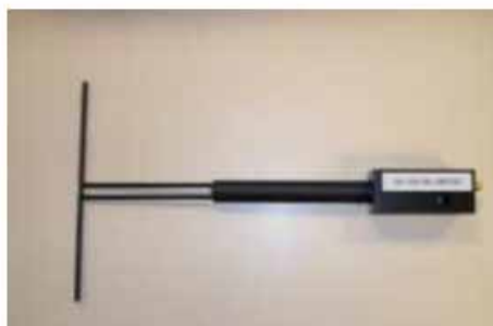
Figure 1 – Satimo COMOSAR Validation Dipole
