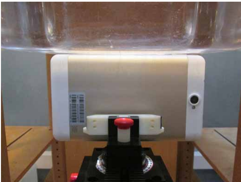
Body-worn Right Setup Photo (0mm)
