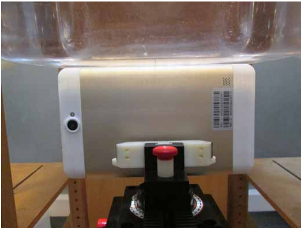
Body-worn Right Setup Photo (0mm)
