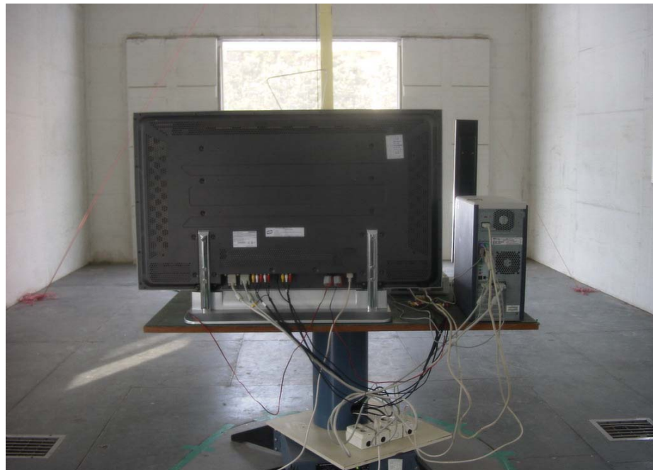
Radiated Emissions 30MHz - 1000 MHz
