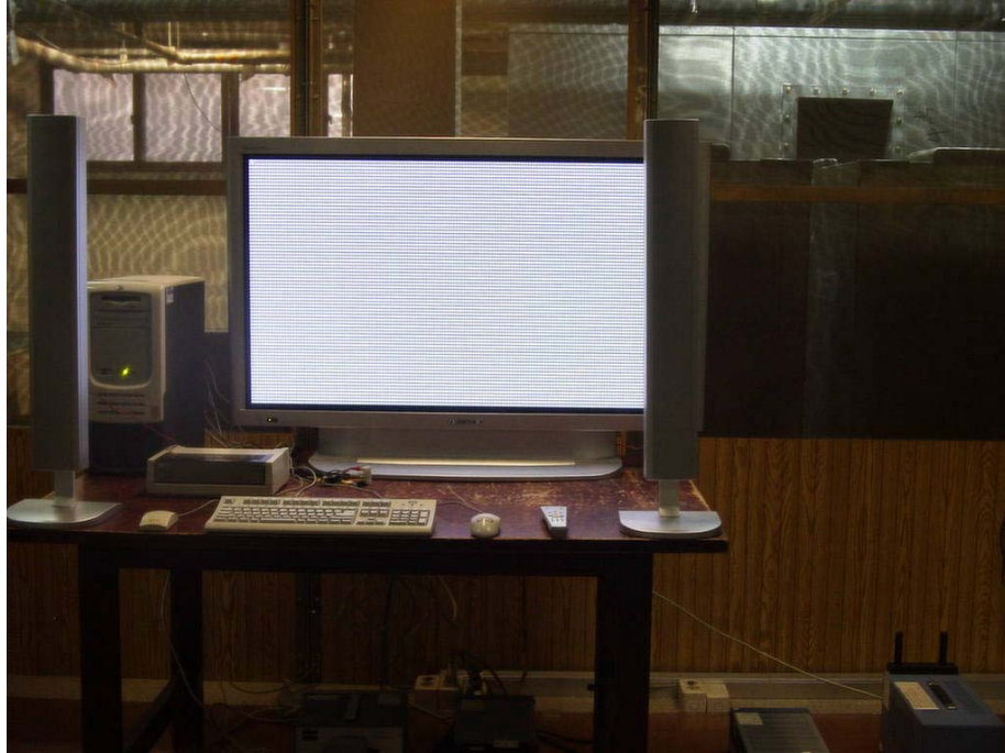
Conducted Emissions 150kHz - 30 MHz
