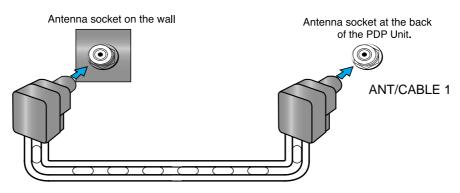
Feeder cable connection with the aombining adapter
