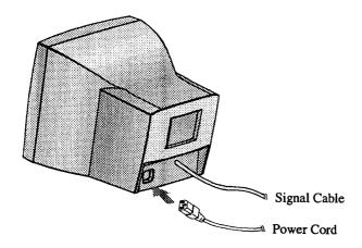
If your power cord is PC-to-Monitor type, plug the other end of the power cord into the AC receptacie in the computer.
