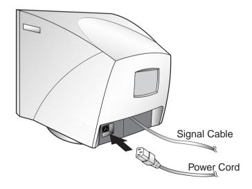
If your power cord is PC-to-Monitor type, plug the other end of the power cord into the AC receptacle in the computer.
