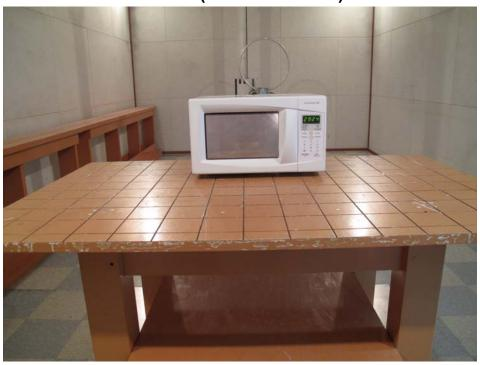
Radiated Test Picture (0.15 MHz~30 MHz)
