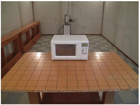
• Radiated Test Picture (0.15 MHz~30 MHz)
