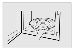
7 The roller guide and oven cavity floor should be cleaned regularly to avoid excessive noise. Simply wipe the bottom surface of the oven with mild detergent water or window cleaner and dry. The roller guide may be washed in mild sudsy water.
