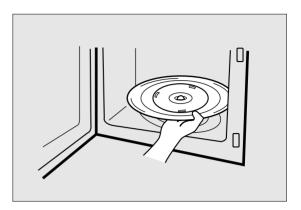
The roller guide and oven cavity floor should be cleaned regularly to avoid excessive noise.
