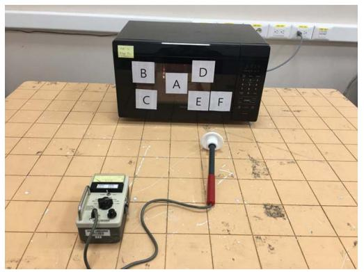
Frequency measurement Test Picture
