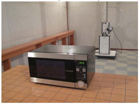
• Radiated Test Picture (0.15 MHz~30 MHz)
