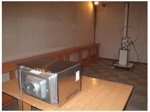
• Radiated Test Picture (0.15 MHz~30 MHz)
