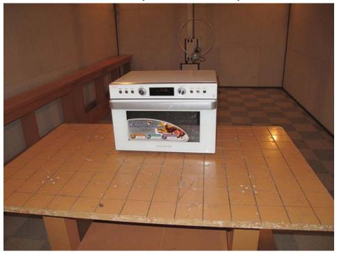
Radiated Test Picture (0.15 MHz~30 MHz)
