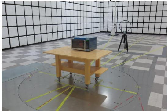
● Radiated Test Picture: 0.15 Mb ~ 30 Mb (Rear)
