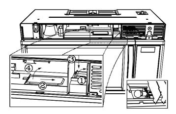
Remove the charcoal filter and pull out the lamp cover. Replace the burned-out bulb with a 30-watt bulb.
