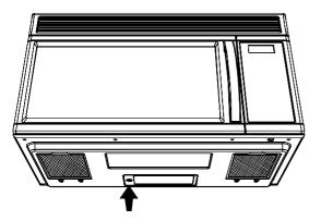
To replace the combination cooktop light/night light, first disconnect power at main fuse or circuit breaker panel or pull plug. Remove screw on right side of light compartment cover and lower cover until it stops.
