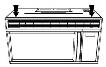
To replace your oven light, first disconnect power at main fuse or circuit breaker panel or pull plug. Remove the top grill by taking out the 2 screws that hold it in place.
