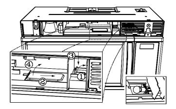
Remove the charcoal filter and pull out the lamp cover. Replace the burned-out bulb with a 30-watt bulb.
