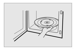
The roller guide and oven cavity floor should be cleaned regularly to avoid excessive noise. Simply wipe the bottom surface of the oven with mild detergent water or window cleaner and dry. The roller guide may be washed in mild sudsy water.
