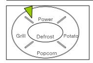
1.change the power level if you don't want full power for cook1.(Press power button. Select a desired power level HI,9  $\sim$  0) the m/w1 indicator lights and  $\boxed{ : 0 }$  is displayed.
