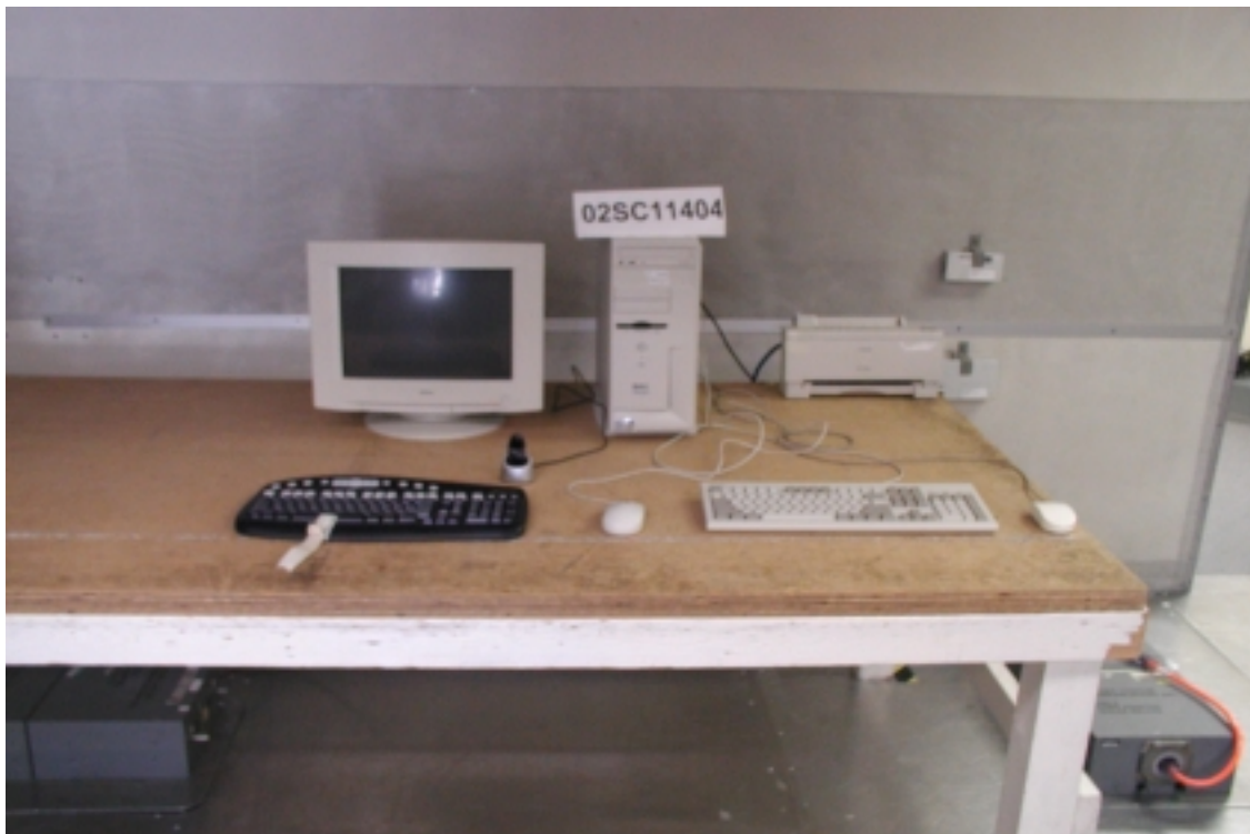
Photo 2 – MS Lapis Conducted Emissions Test Setup
