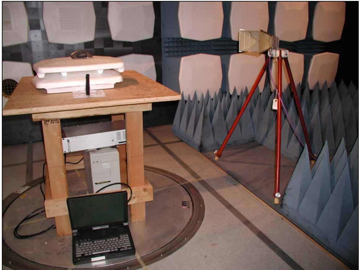
Photo 1 – EUT Bluetooth Test Set -1m High – 1m from Horn 1-18GHz Testing
