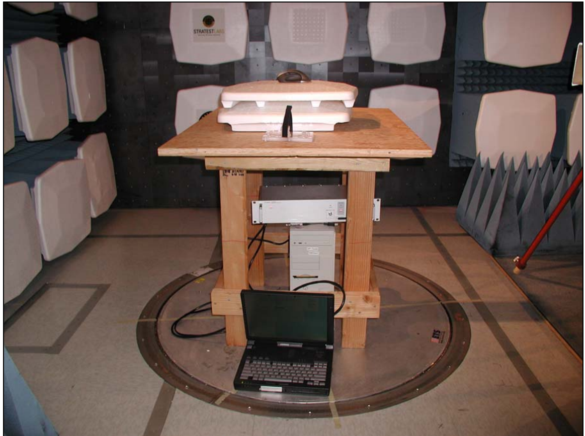
Photo 2 – Picture of EUT Test Configuration – 1-18GHz Testing
