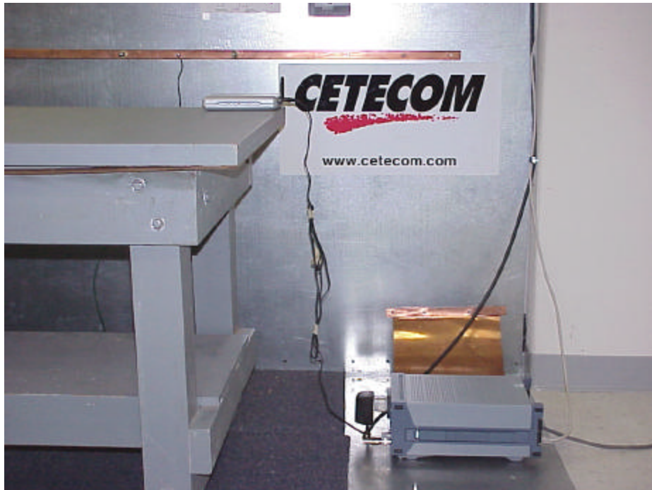
Test setup – AC Line conducted emissions
