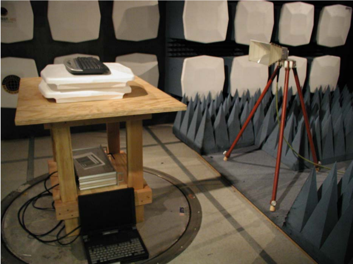
Photo 1 – MS Azure Keyboard with Bluetooth Test Set - 1m High – 1m from Horn
