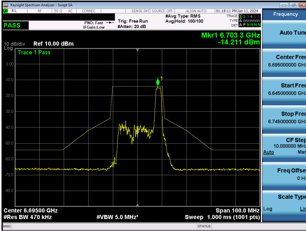
Plot 7-316. In-Band Emission Plot MIMO ANT2 (20MHz BW 802.11be (26 Tones) (UNII Band 7) – Ch. 149) - LPI
