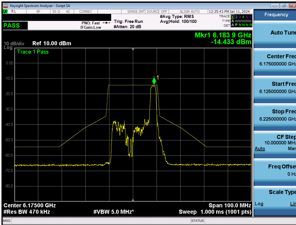
Plot 7-306. In-Band Emission Plot MIMO ANT2 (20MHz BW 802.11be (26 Tones) (UNII Band 5) – Ch. 45) - LPI
