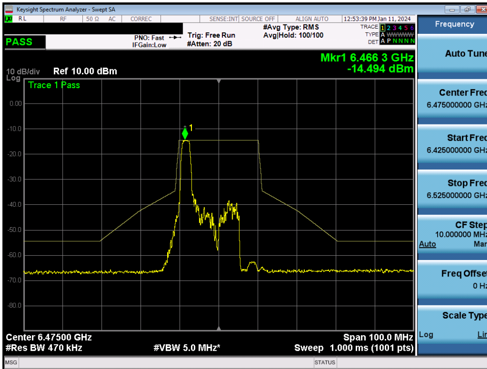
Plot 7-311. In-Band Emission Plot MIMO ANT2 (20MHz BW 802.11be (26 Tones) (UNII Band 6) – Ch. 105) - LPI
