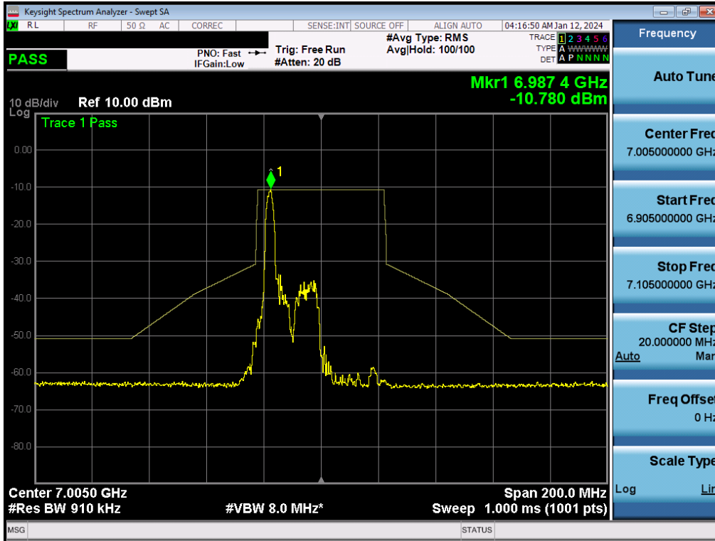
Plot 7-322. In-Band Emission Plot MIMO ANT2 (40MHz BW 802.11be (26 Tones) (UNII Band 8) – Ch. 211) - LPI
