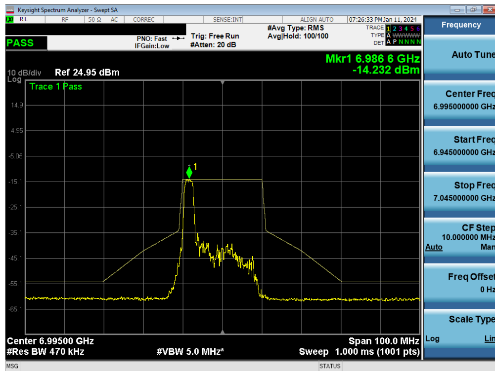
Plot 7-246. In-Band Emission Plot MIMO ANT1 (20MHz BW 802.11be (26 Tones) (UNII Band 8) – Ch. 209) - LPI
