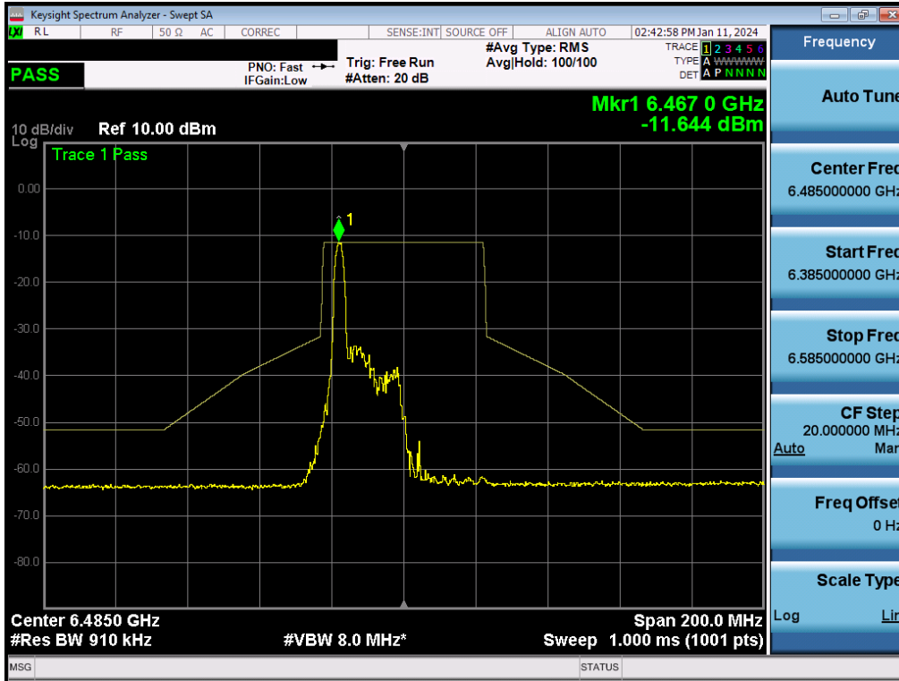
Plot 7-312. In-Band Emission Plot MIMO ANT2 (40MHz BW 802.11be (26 Tones) (UNII Band 6) – Ch. 107) - LPI
