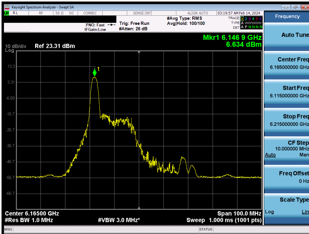
Plot 7-209. Power Spectral Density Plot MIMO ANT2 (40MHz BW 802.11be (26 Tones) (UNII Band 5) – Ch. 43) - SP
