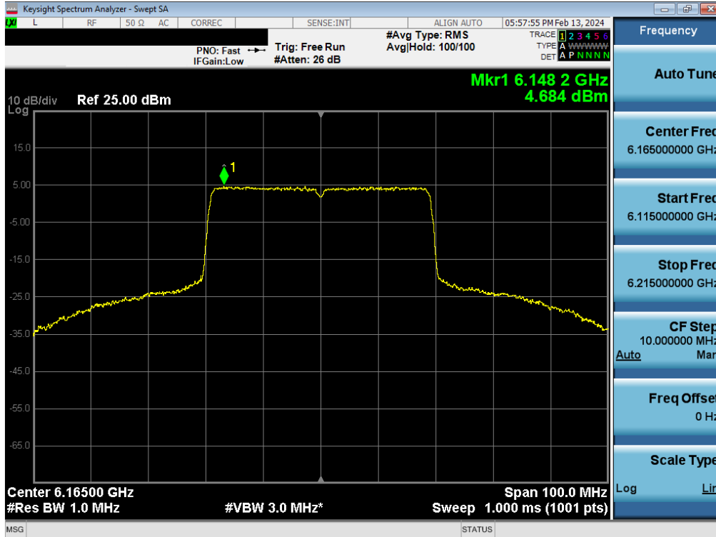
Plot 7-143. Power Spectral Density Plot MIMO ANT1 (40MHz BW 802.11be (Full Tones) (UNII Band 5) – Ch. 43) - SP
