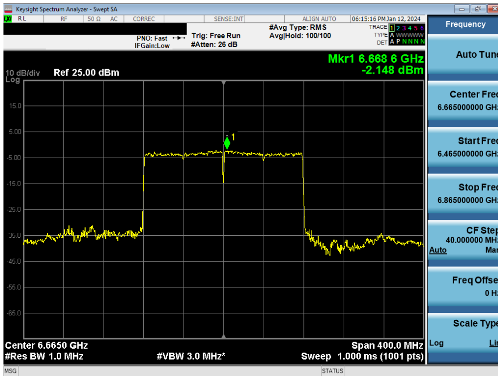
Plot 7-150. Power Spectral Density Plot MIMO ANT1 (160MHz BW 802.11be (Full Tone) (UNII Band 7) – Ch. 143) – SP
