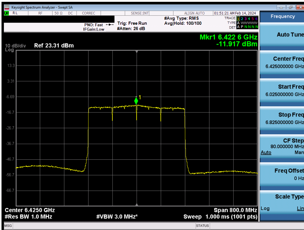
Plot 7-185. Power Spectral Density Plot MIMO ANT2 (320MHz BW 802.11be (Full Tone) (UNII Band 6) – Ch. 95) – LPI
