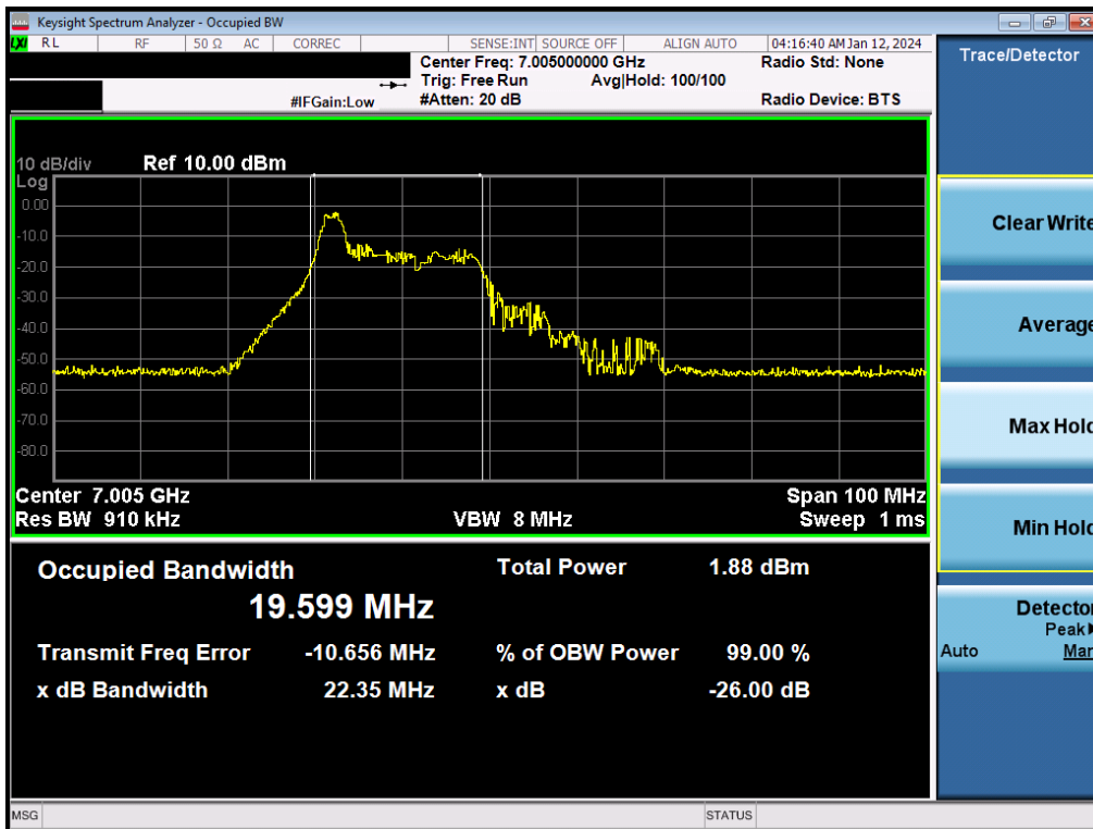
Plot 7-57. Occupied Bandwidth Plot MIMO ANT2 (40MHz BW 802. 11be (26 Tones) (UNII Band 8) – Ch. 211)
