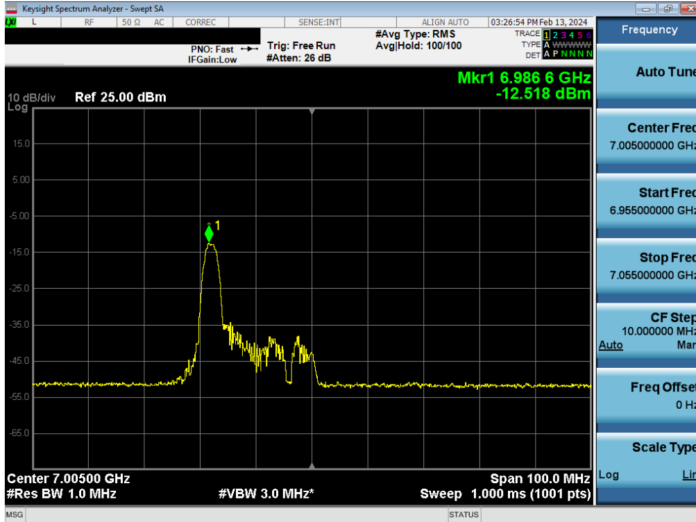
Plot 7-97. Power Spectral Density Plot MIMO ANT1 (40MHz BW 802.11be (26 Tones) (UNII Band 8) – Ch. 211) - LPI
