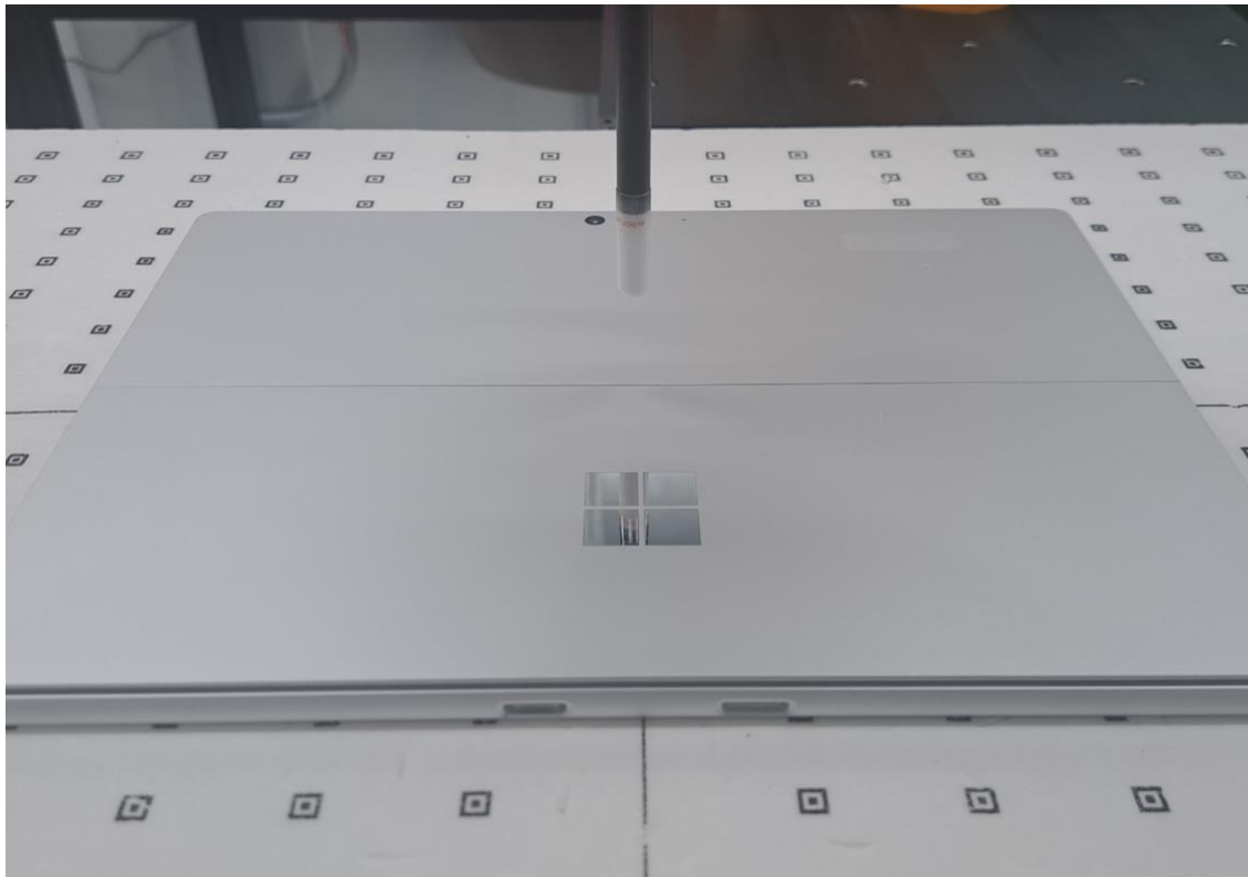
PD Test Setup Photo 28 – Near Field Power Density Back Side at 25 mm
