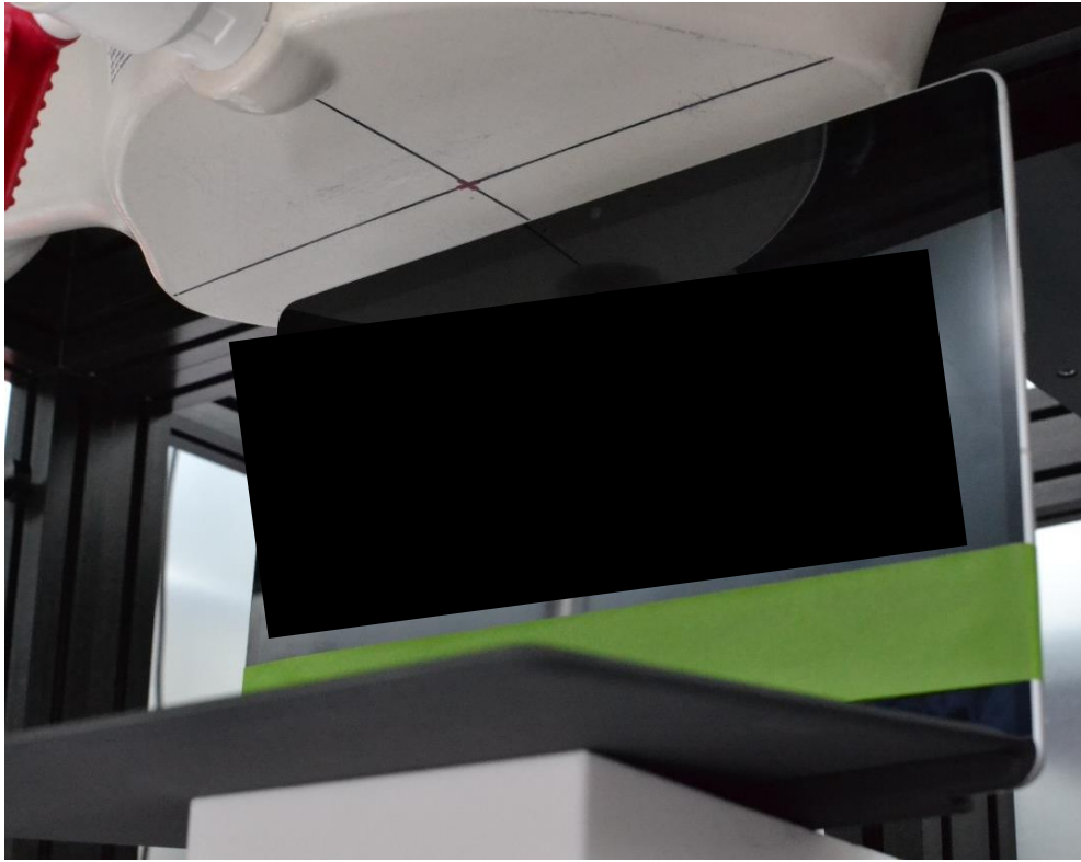
SAR Test Setup Photo 12 – Laptop, Top Edge at 25mm – Antenna L
