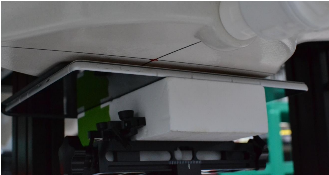
SAR Test Setup Photo 5 – Tablet with keyboard accessory, Back Side at 0mm – Antenna L
