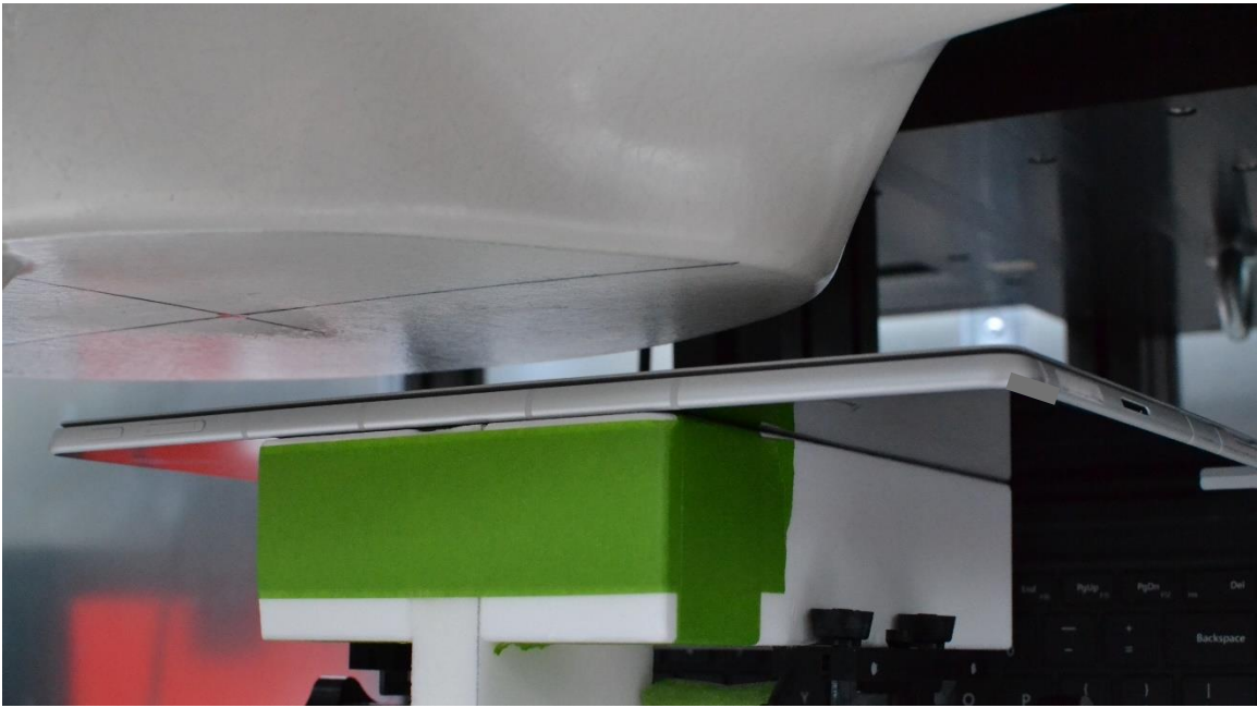
SAR Test Setup Photo 6 – Laptop, Back Side at 25mm – Antenna L
