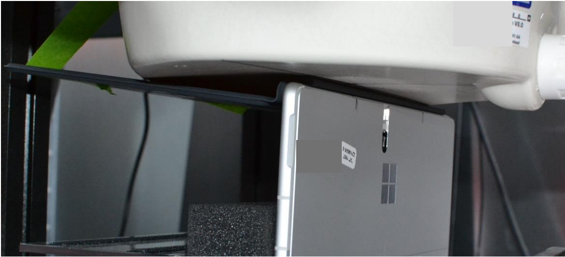
SAR Test Setup Photo 17 – Laptop, Bottom Edge at 0mm – Antenna L
