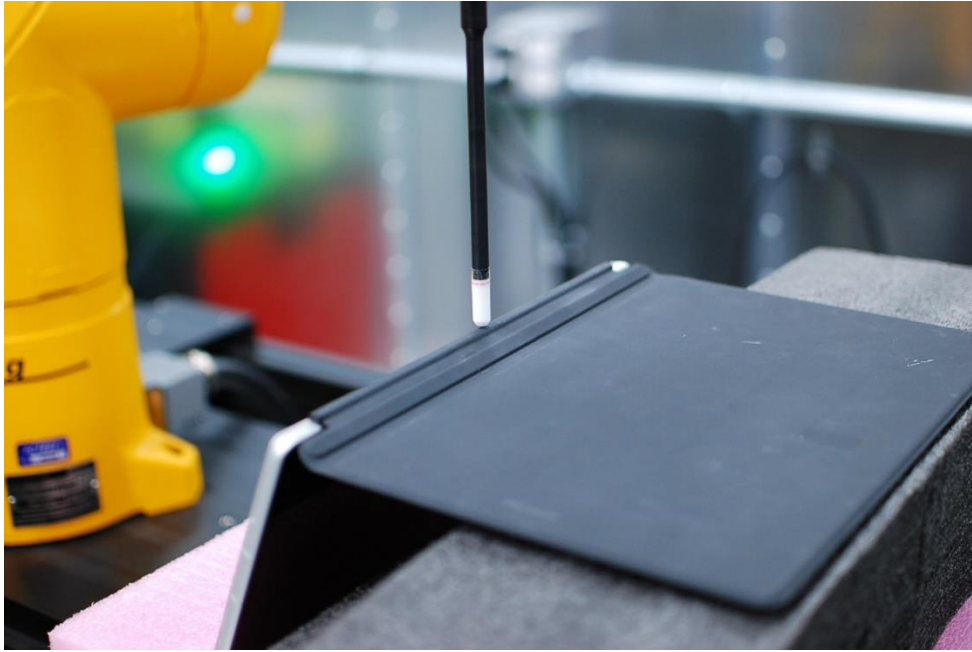
PD Test Setup Photo 34 – Near Field Power Density Laptop Bottom Edge at 2 mm
