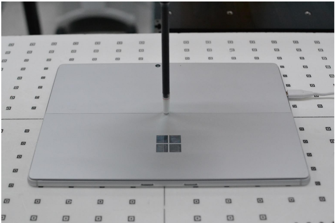
Test Setup Photo 27 – Near Field Power Density Back Side at 2 mm
