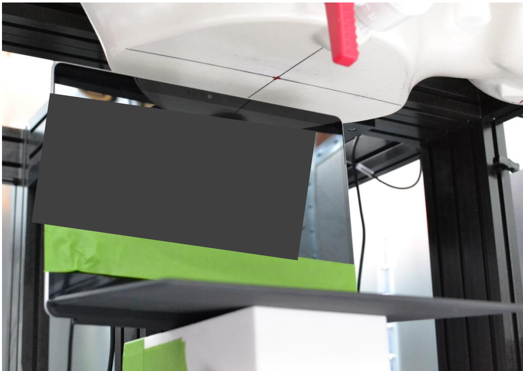
SAR Test Setup Photo 9 – Laptop, Top Edge at 25 mm – Antenna R
