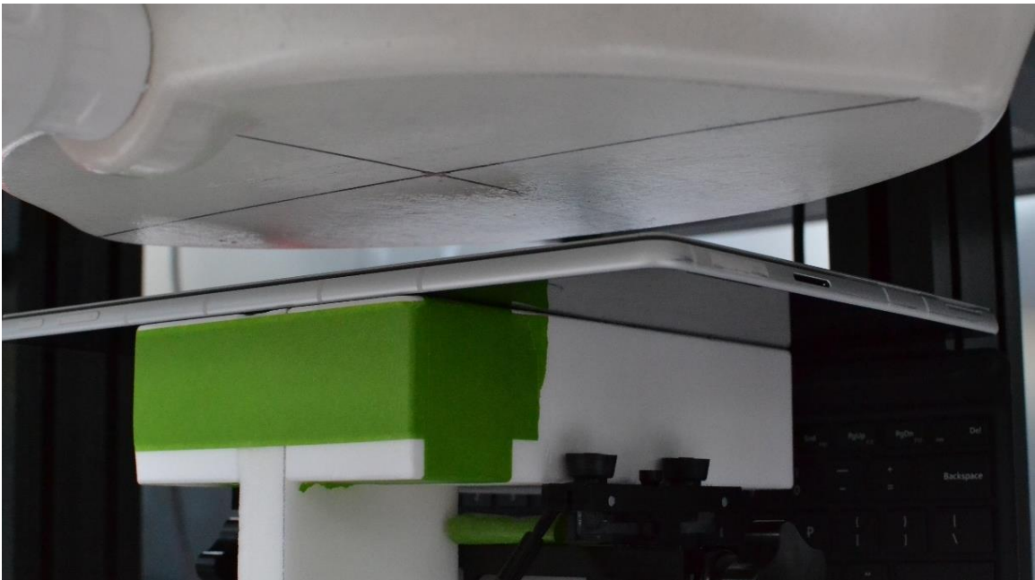
SAR Test Setup Photo 2 – Laptop, Back Side at 25 mm – Antenna R
