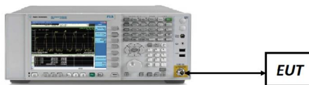
Figure 7-4. Test Instrument & Measurement Setup
