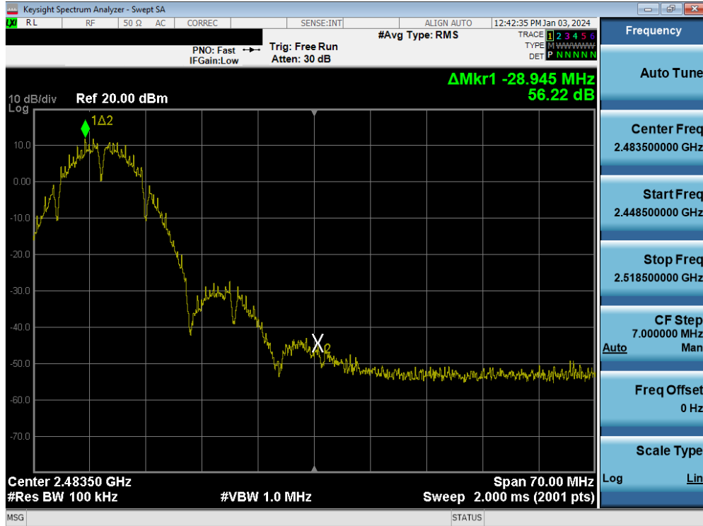
Plot 7-75. Band Edge Plot MIMO ANT1 (802.11b – Ch. 10)
