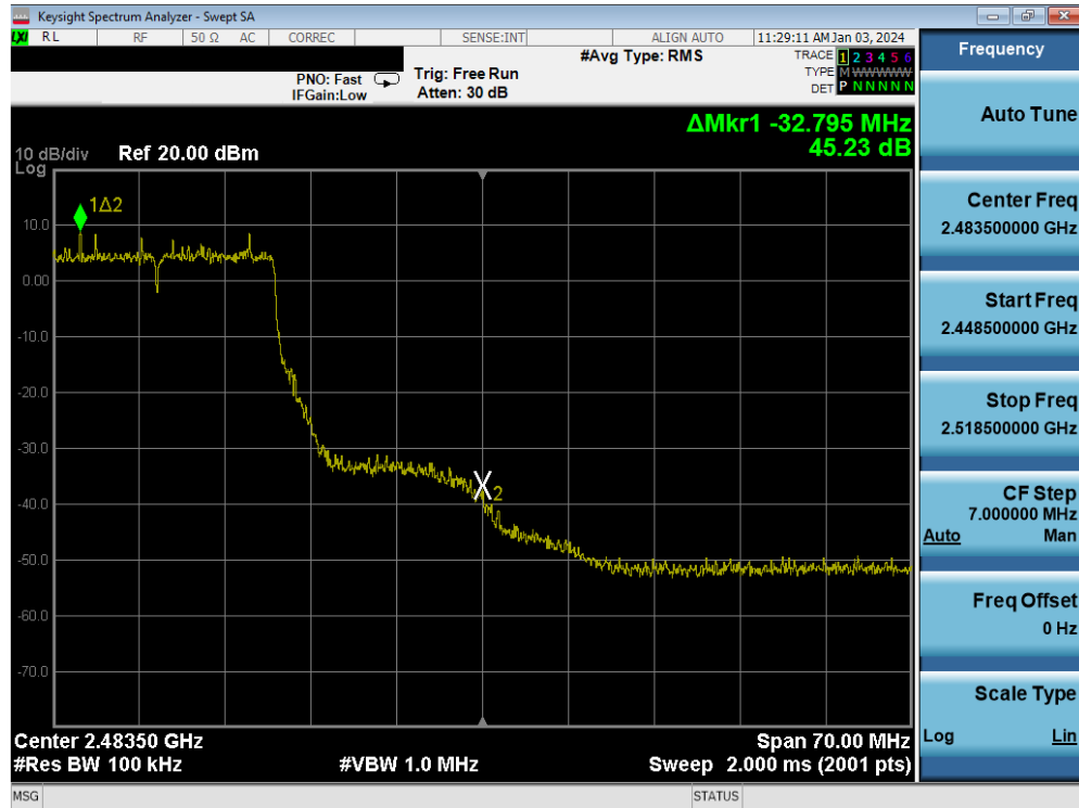
Plot 7-94. Band Edge Plot MIMO ANT1 (802.11be (2.4GHz) – Ch. 10)
