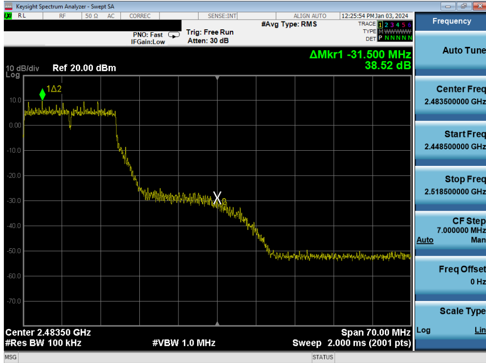
Plot 7-106. Band Edge Plot MIMO ANT2 (802.11g – Ch. 10)
