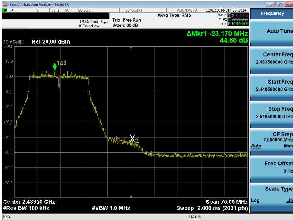
Plot 7-88. Band Edge Plot MIMO ANT1 (802.11n (2.4GHz) – Ch. 11)
