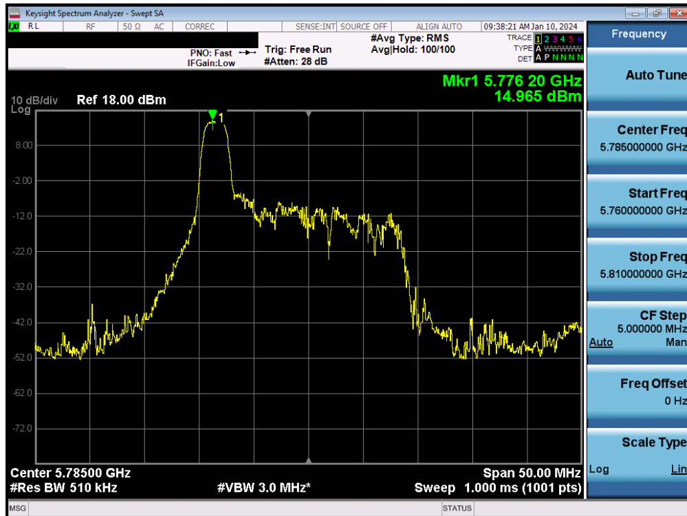
Plot 7-138. Power Spectral Density Plot MIMO ANT2 (20MHz BW 802.11be – 26 Tones (UNII Band 3) – Ch. 157)
