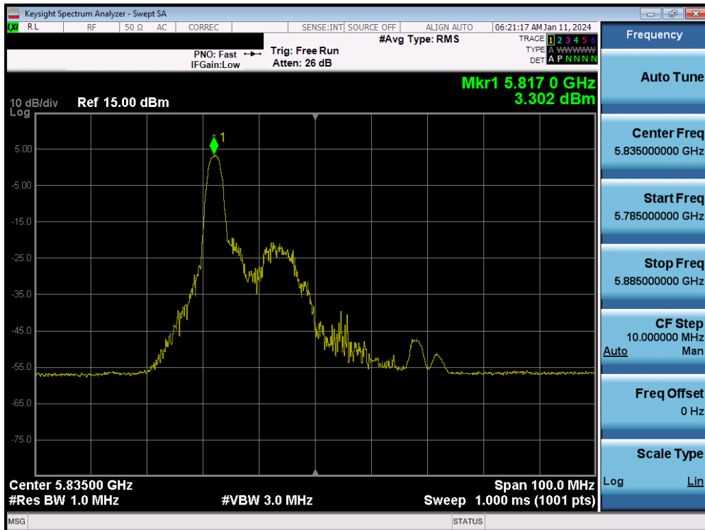
Plot 7-142. Power Spectral Density Plot MIMO ANT2 (40MHz BW 802.11be – 26 Tones (UNII Band 3/4) – Ch. 167)
