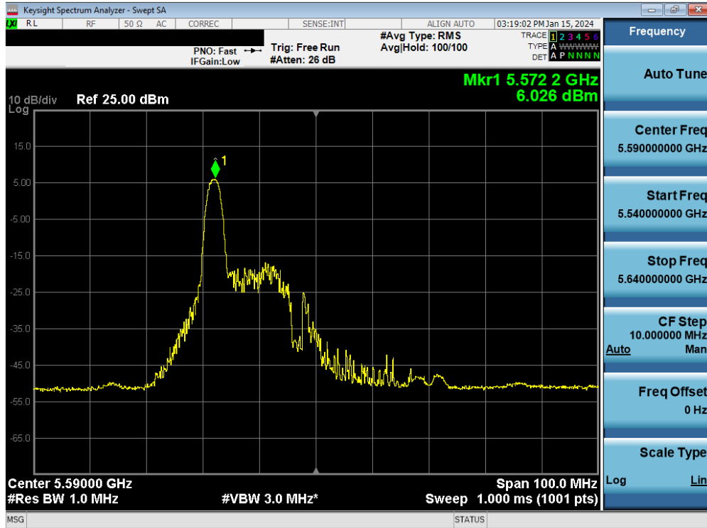
Plot 7-81. Power Spectral Density Plot MIMO ANT1 (40MHz BW 802.11be – 26 Tones (UNII Band 2C) – Ch. 118)
