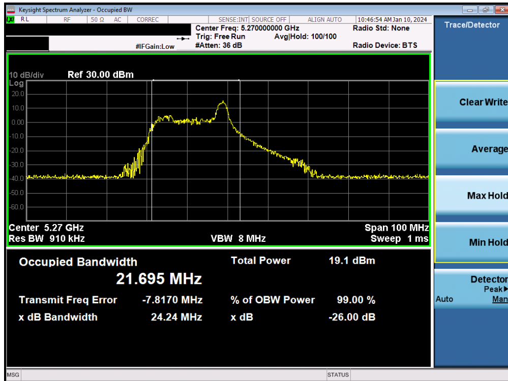
Plot 7-28. 26dB Bandwidth Plot MIMO ANT2 (40MHz BW 802.11be – 26 Tones (UNII Band 2A) – Ch. 54)
