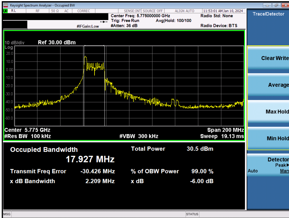
Plot 7-61. 6dB Bandwidth Plot MIMO ANT2 (80MHz BW 802.11be – 26 Tones (UNII Band 3) – Ch. 155)
