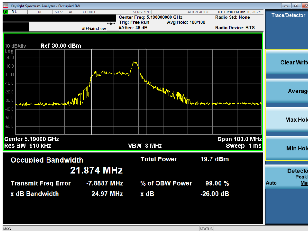
Plot 7-2. 26dB Bandwidth Plot MIMO ANT1 (40MHz BW 802.11be – 26 Tones (UNII Band 1) – Ch. 38)
