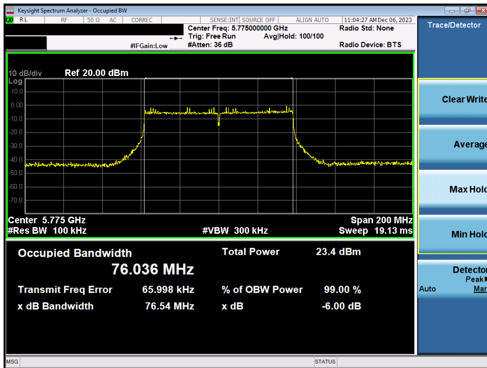
Plot 7-56. 6dB Bandwidth Plot MIMO ANT1 (80MHz BW 802.11ac (UNII Band 3) – Ch. 155)
